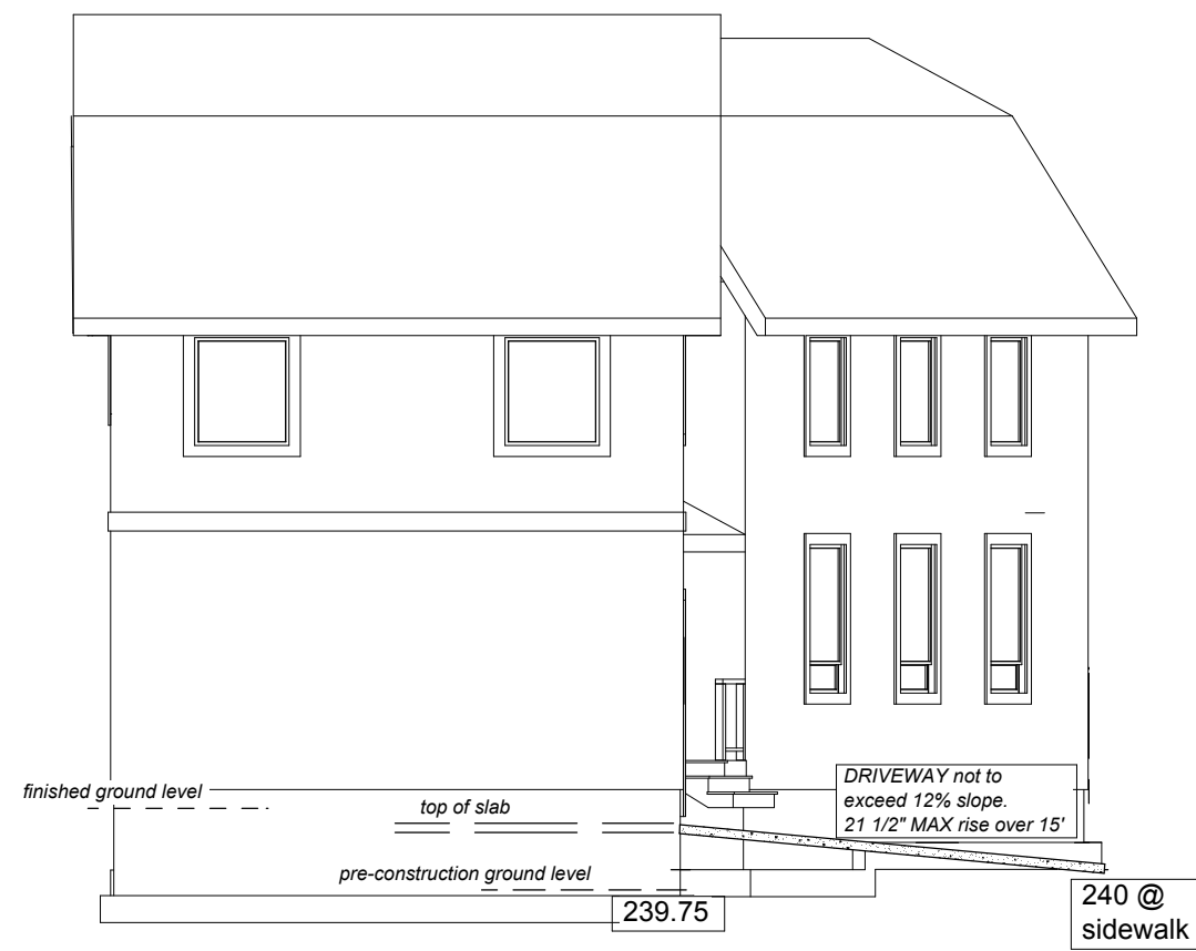
DRIVEWAY SLOPE Scale: 1/8" = 1'
